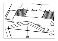
hands on the metal contacts on the handgrip pulse sensor. Your palms should be resting on the upper contacts and your fingertips should be touching the lower contacts. **Avoid moving your hands**. When your pulse is detected, two dashes (--) will appear in the Pulse/Calories/Fat Calories display, and then your heart rate will be shown. For the most accurate heart rate reading, continue to hold the contacts for about 15 seconds.
